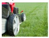
A rotary mower slings off the grass because the blade in the mower rotates quickly. This makes the grass a bit rougher. When mowing, take care of stones, twigs or other waste that might get slung away at high speed; avoid contact as much as possible. Like the cage mower, the blade of the rotary mower must be sharpened every year for a good result.
