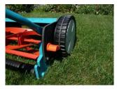
A cage mower is used to cut the grass short. This mower cuts the grass, resulting in cleaner cut grass. However, a cage mower suffers from more wear than a rotary mower and thus requires more maintenance.
